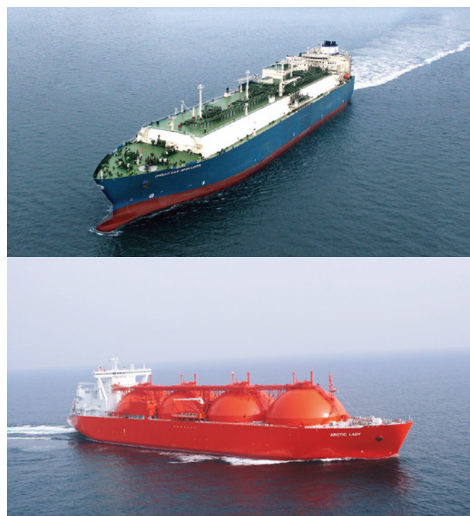
Figure 4. Examples of LNG carrier types: membrane design (top); Moss sphere design (bottom)
