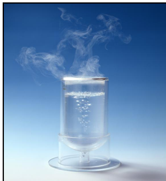
Figure 1. LNG “boiling” at atmospheric pressure and temperature (Source: OSAKA Gas Co. Ltd.)
