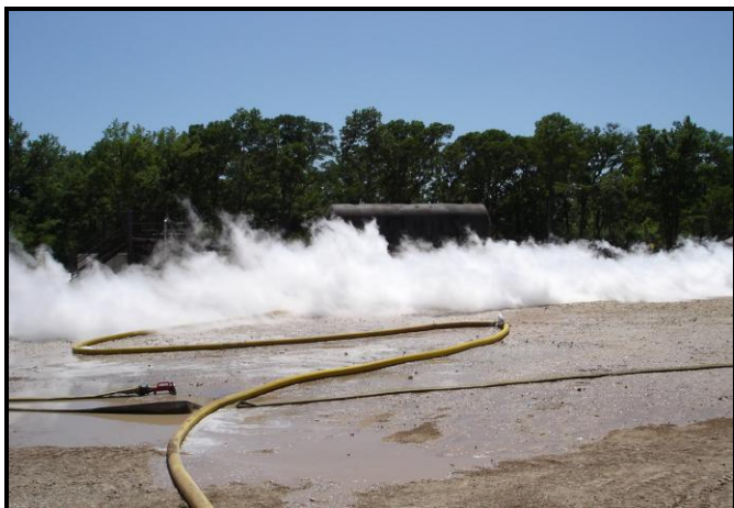
Figure 2. LNG vapour cloud created for training at Texas A&M in the LNG Live Fire Training Workshop (2005) (Photograph by A.H. Walker)
