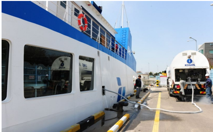
Truck-to-Ship LNG bunkering for ECONURI by KOGAS at Incheon port
