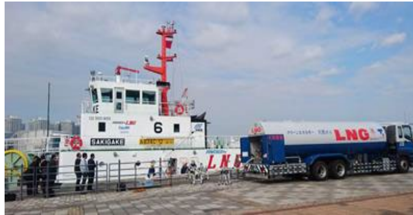
Truck-to-Ship LNG bunkering for Sakigake by Tokyo Gas at Yokohama port
