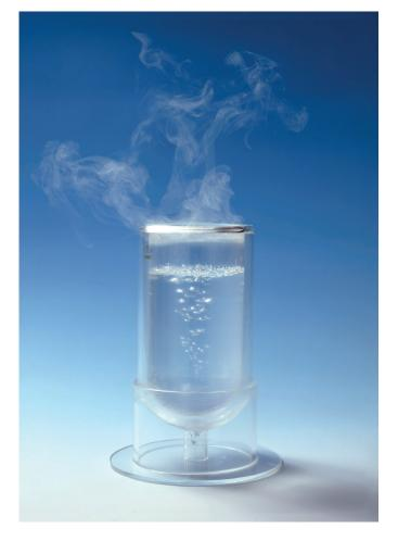
Figure 1. LNG "boiling" at atmospheric pressure and temperature (Source: OSAKA Gas)
