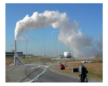
Figure 2. LNG Vapour Cloud created at ENGIE Lab CRIGEN LNG testing facility (Source: Engie Lab)
