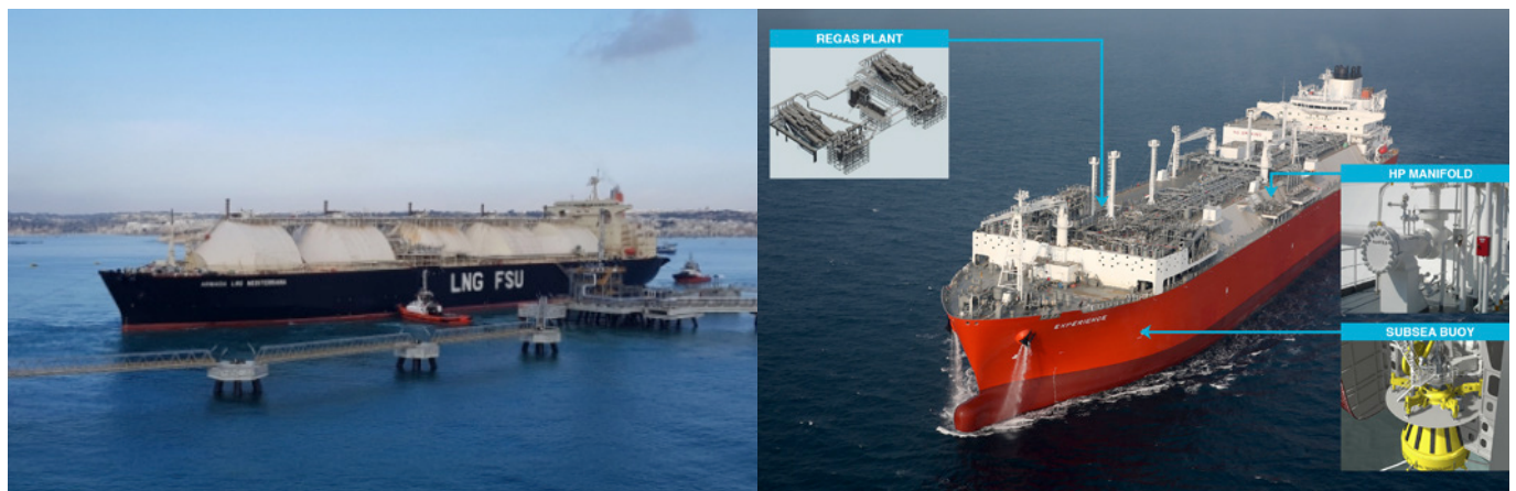
Figure 2. Floating facilities: FSU (Left) and FSRU (Right) (Source: Reganosa, Excelerate LNG)
