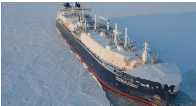
Figure 3. Christophe de Margerie - the world's first icebreaking LNG carrier (Source: DSME)
