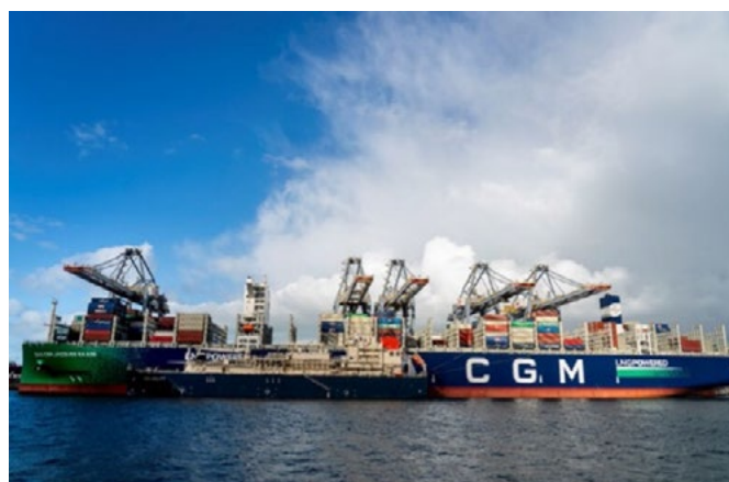
LNG Bunkering Vessel alongside a large container vessel (Source: Rotterdam port)
