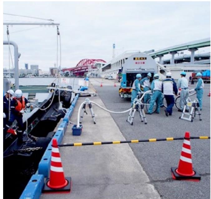
LNG bunkering to a tugboat (Source: MOL)
